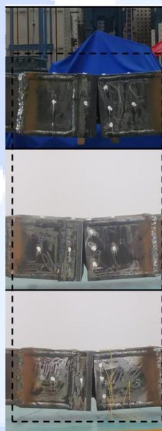
Figure 4. Vertical plate failure (Zhang et al. 2024 [8])
