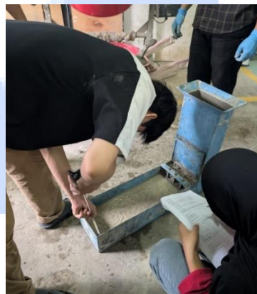
Figure 4. L-box test setup for evaluating the passing ability of fresh SCC
