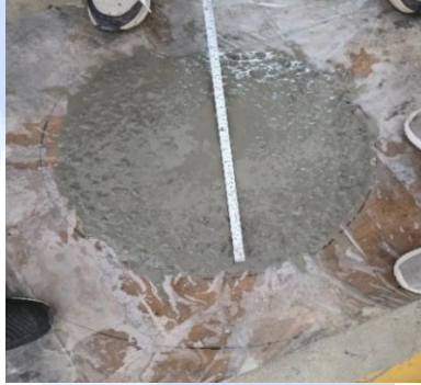
Figure 2. Slump flow test setup for evaluating the filling ability of fresh SCC
