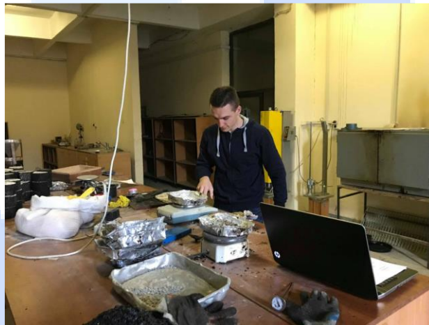
Figure 3. Laboratory preparation and weighing of aggregate fractions for the Marshall specimens
