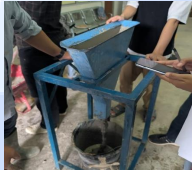
Figure 3. V-funnel test setup for evaluating the viscosity of fresh SCC
