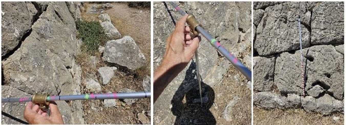
Figure 7. Measurements by the T-FORM GEOMETRY TOOL. The COLOURED Regions of the SLOPES' NUMBER shown
