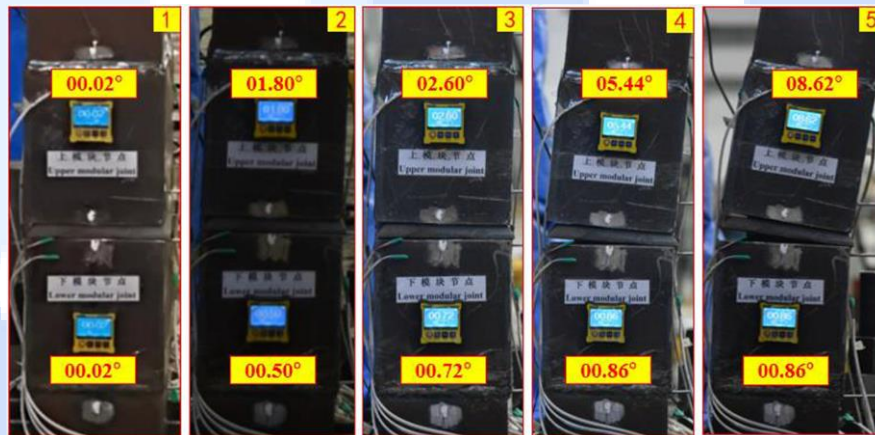
Figure 7. Rotational stiffness testing (Chen et al. 2019) [10]
